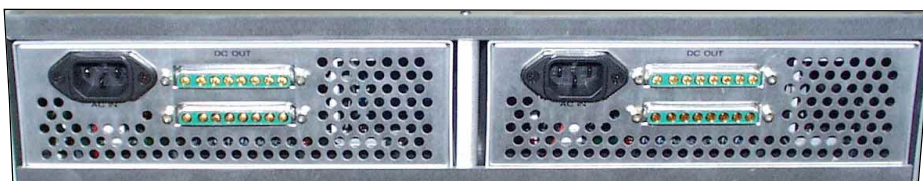
Rear view of the PSR (SPS-40) rackmount power supply
